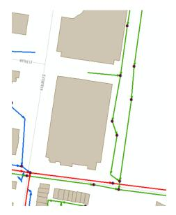
Response: Applicant has explored a parallel system adjacent to the existing sewer and this sewer will only carry flows from the PRGS site to tie into the existing sewer line at N. First Street, east of the N. Fairfax St. Further refinement will occur in Final IDSP. This 27" line has been shown on sheets C700-C702.
